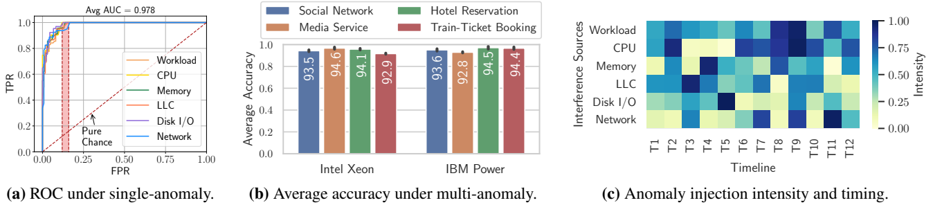
Figure 9: Critical Component Localization Performance: (a) ROC curves for detection accuracy; (b) Variation of localization accuracies across processor architectures; (c) Anomaly-injection intensity, types, and timing.
